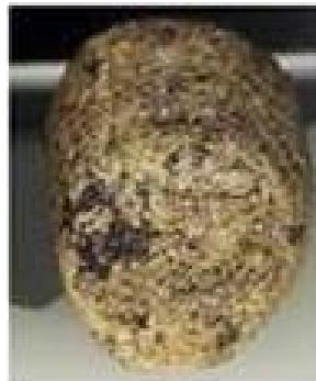
Consumed permanganate wax cylinder
